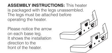
1. Insert the protrusions on the leg into the notches on the bottom of the heater.
